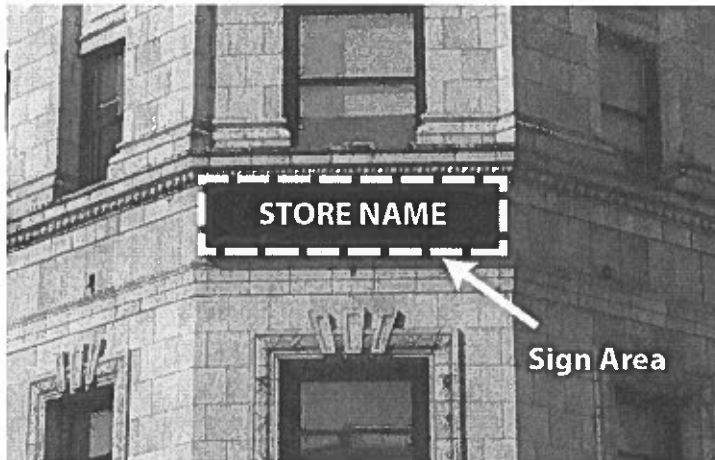
Figure B: Illustration of computing the sign area for wall signs with a background panel or cabinet.
